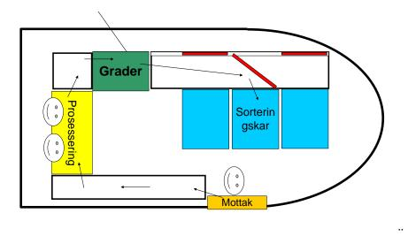
Figure 1. Typical installation of a grader on a high seas fishing vessel.
