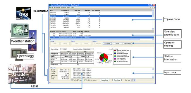
Figure 2. Operating panel from the programme Datafangst, with illustration of possible instruments that could be connected.
