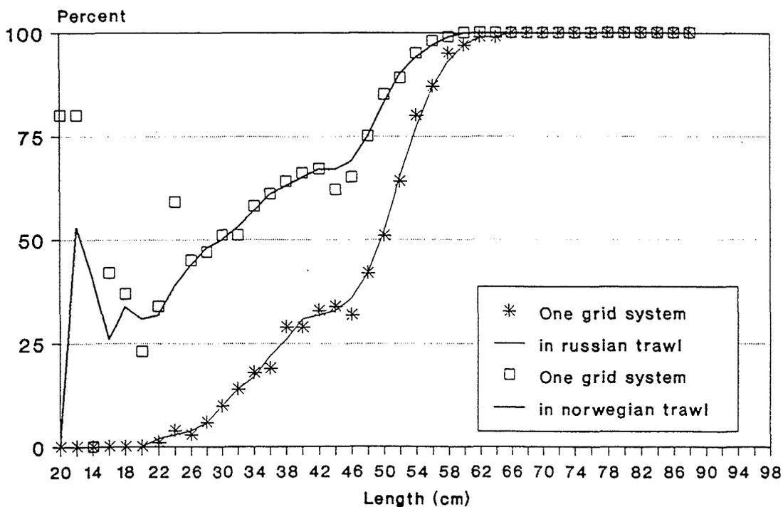
Figure 7. Selection curves for cod when using the one-grid sorting system in both the Norwegian and the Russian types of trawl.
