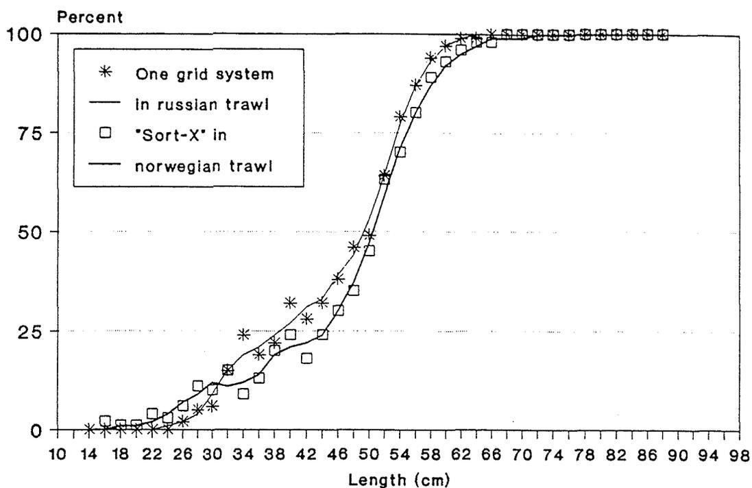
Figure 6. Selection curves for cod when using the "Sort-X" system in Norwegian trawl (Alfredo type) and the single-grid system in the Russian trawl.
