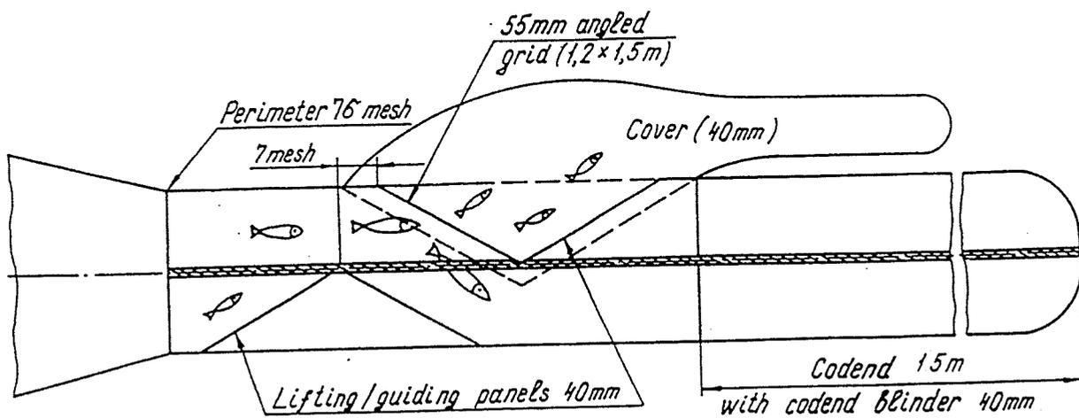
Figure 4. Illustration of cover used to collect fish that have escaped through the "Sort-V" single-grid sorting system.
