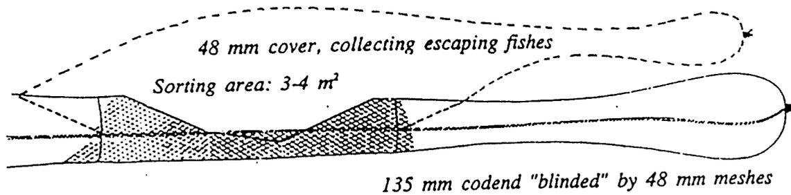
Figure 3. Illustration of cover used to collect fish that have escaped through the "Sort-X" grid-sorting system.
