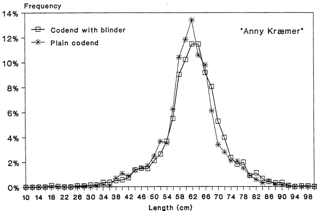
Figure 10. Length frequency distribution of cod when fishing with 55 mm inter-bar distance and codend with or without blinder. ("Anny Kræmer" with "Sort-X" and 52 mm codend blinder or plain 137 mm codend, "Bizon" with single-grid sorting system and 60 mm codend blinder or plain 137 mm codend, both boats with Norwegian type codend material, see Table 1).
