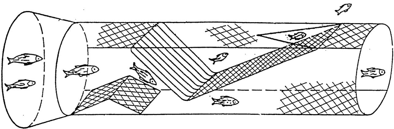
Figure 2. Illustration of the working principle of the single-grid system ("Sort-V", PINRO construction) in a bottom trawl.
