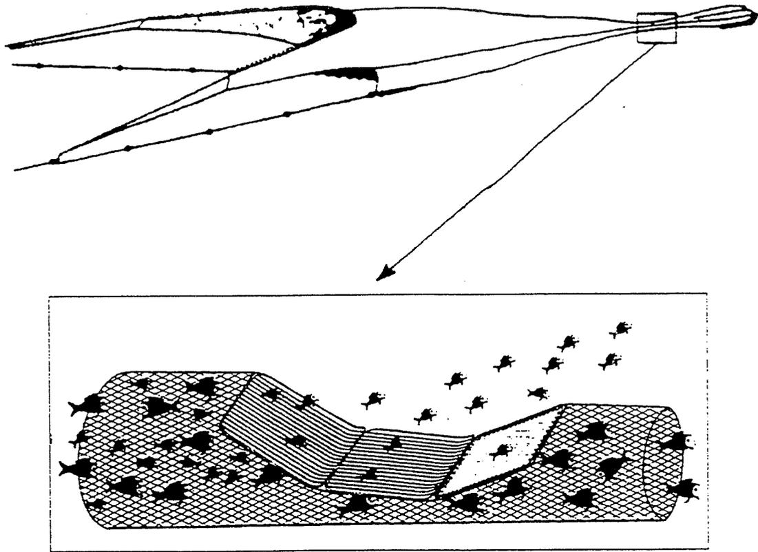
Figure 1. Illustration of the location and working principle of the sorting grid system "Sort-X" in a bottom trawl.
