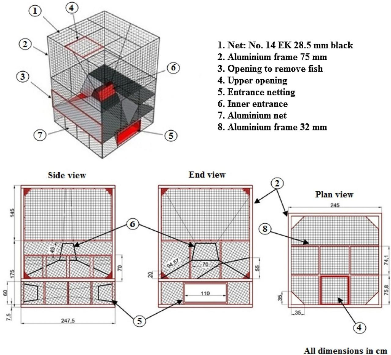
Fig. 2. Design of the rigid pot tested in the fishing trials.
