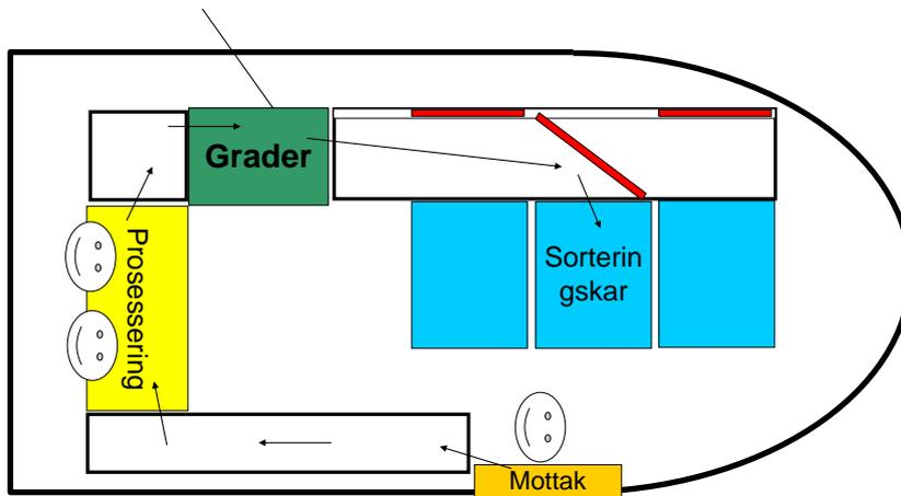
Figure 1. Typical installation of a grader on a high seas fishing vessel.
