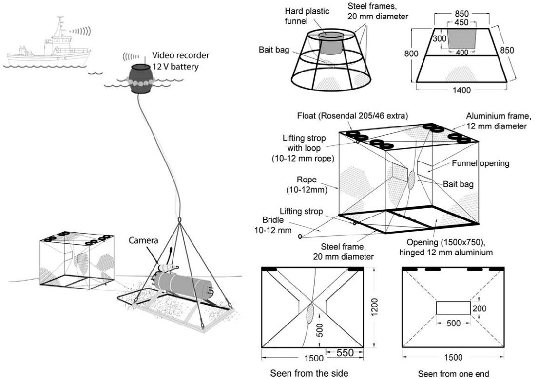
FIGURE 1.—Experimental setup used to study the search behavior of red king crabs vis-à-vis baited square and conical pots. Design details are given in the right-hand portion of the figure. Dimensions are in millimeters.
