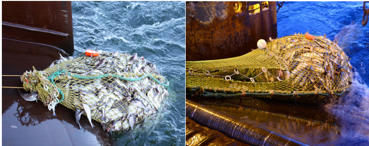
Fig. 5. Photographs showing a semi-detached codend (left) and a codend with side splits (right) being hauled on board the fishing vessel.
